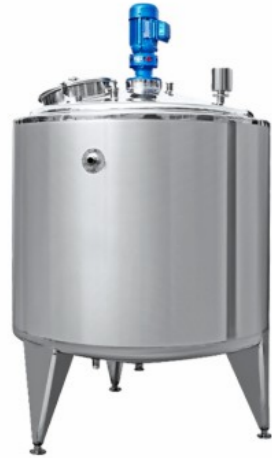
调配罐 Blending tank
